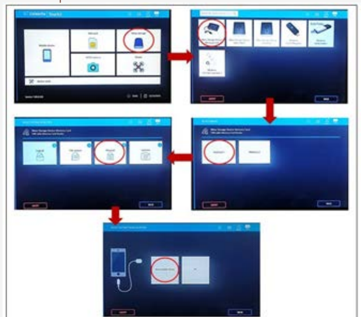
Figure 4: Steps involved in the extraction of data from Memory Card
