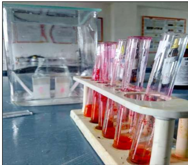
Figure 6: Red Ink Samples collected in test tube by dissolving 3ml of Methanol
